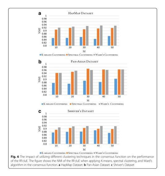
40, 50}, *ntrees* = 10000,  $MN = \sqrt{N}$ , and  $k = \sqrt{N}$ ). We can see that Ward's clustering, applied with RFcluE, has the best performance compared with K-means and spectral clustering across all the examined datasets, demonstrating statistically significant performance, with a *p*-value < 0.05.
